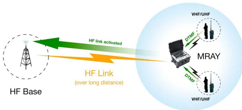
**MRAY Solution:** The field personnel deploy an MRAY transportable radio and use the HF link to communicate back to the command center. The command center can use an HF radio (or an MRAY) to create a link to the field personnel (via the MRAY) over long distance. The field personnel do not require HF radio equipment to communicate back with the command center, using less expensive and smaller LMR handheld radios.
